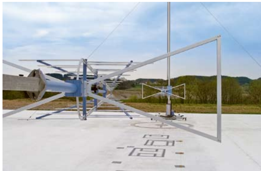
ULTRALOG R&S® HL 562 at open-area test site
